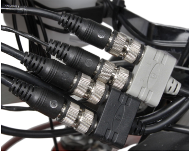
Gray splitter for temperature and black for receiver and speed.
