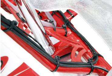
Cable fixed to frame. Run RPM wire separately.
