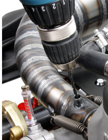
Drill a \varnothing 4.5 mm hole for the sensor through the exhaust fitting.
