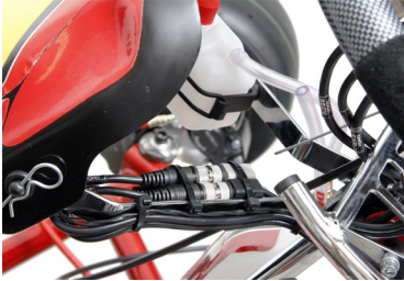
Two splitters mounted to increase number of sensors.
