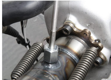
Exhaust fitting welded on the exhaust pipe.
